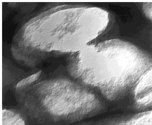
Figure 11 TEM micrograph of the PMBT/PBD-NH 2 latex film. The PMBT particle size was 280 nm. The black area is the PBD-NH 2 (stained by osmium tetroxide). The bright area is the PMBT. The gray area is the PMBT/PBD-NH 2 interphase.
